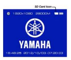
After installing the SD card, power on the camera and an SD card icon will appear in the top right corner of the screen – this indicates SD card is correctly installed. If no icon is displayed then an SD card is not installed or the card is invalid.
